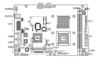
Figure 2.1: EX-98211 Main Board Top View
